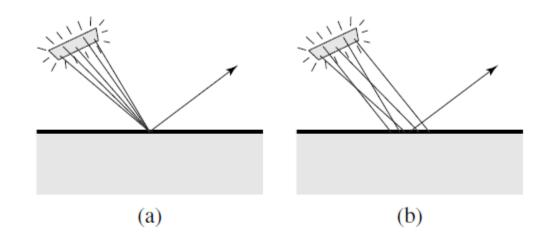
Figure 7: (a) Sampling a BRDF (traditional sampling), (b) sampling a BSSRDF (the sample points are distributed both over the surface as well as the light).
