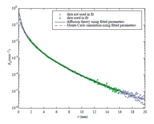
Figure 6: Measurements for marble (green wavelength band) plotted with fit to diffusion theory and confirming Monte Carlo simulation.
