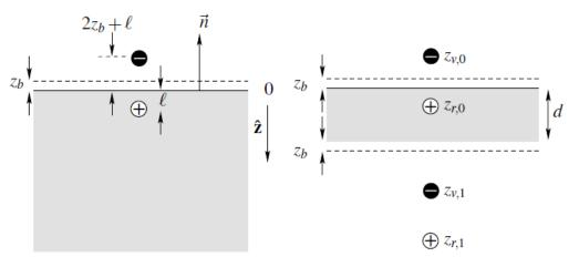
Figure 1: Dipole configuration for semi-infinite geometry (left), and the multipole configuration for thin slabs (right).
